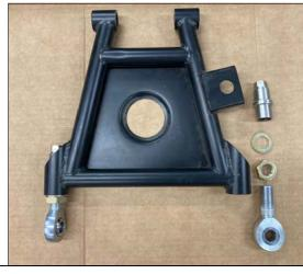
The adjustable A-arms shown in the photos above were not fabricated from details presented in this set of drawings. The photos are provided to show a completed set of adjustable A-arms utilizing the basic adjustment concept and A-arm modifications that are required.
